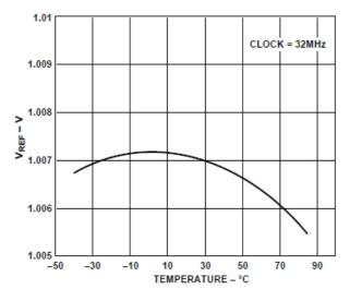
Figure 9. Voltage Reference Error vs. Temperature
