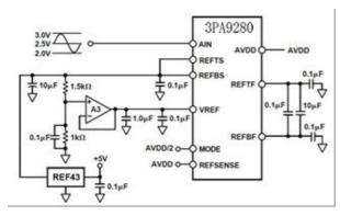
Figure 21. External Reference Mode—1 V p-p Input Span 2.5 VCM
