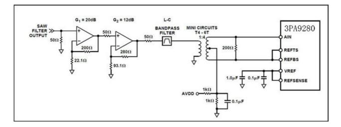
Figure 31. Simplified 3PA9280 IF Sampling Circuit
