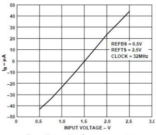
Figure 14. Input Bias Current vs. Input Voltage
