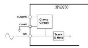
Figure 22c, DC-coupled input
