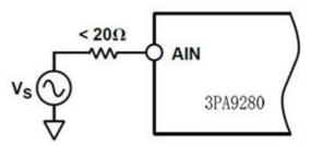
Figure 24. Simple 3PA9280 Drive Configuration
