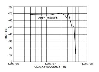
Figure 8. THD vs. Clock Frequency
