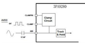
Figure 22a, Bottom signal level clamped to CLAMPIN
