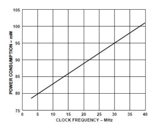
Figure 10. Power Consumption vs. Clock Frequency (MODE = AVSS)
