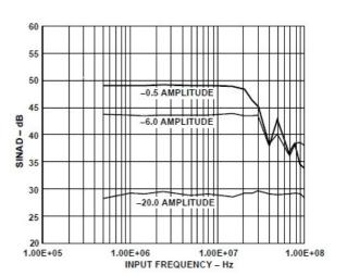
Figure 6. SINAD vs. Input Frequency
