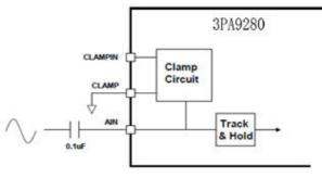
Figure 22b, Bottom signal level clamped to ground
