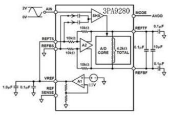
Figure 20 shows the single-ended configuration that gives the good high frequency dynamic performance (SINAD, SFDR). To optimize dynamic performance, center the common-mode voltage of the analog input at approximately 1.5 V. Connect the shorted REFTS and REFBS inputs to a low impedance 1.5 V source. In this configuration, the MODE pin is driven to a voltage at midsupply (AVDD/2). Maximum reference drive is 1 mA. An external buffer is required for heavier loads.
