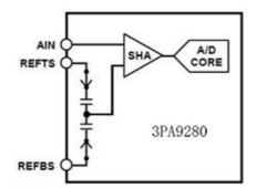
Figure 15. 3PA9280 Equivalent Functional Input Circuit
