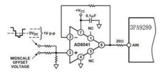
Figure 26. Bipolar Level Shift
