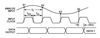
Figure 28. Timing Diagram
