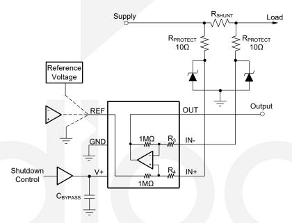
Figure 15. DIO2399x Transient Protection Using Dual Zener Diodes
