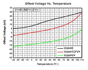
Figure 4. Offset Voltage Vs. Temperature (DIO2399A: 50V/V)
