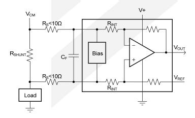
Figure 12. Filter at Input Pins
