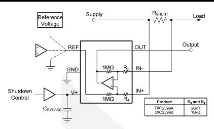
Figure 13. Basic Circuit for Shutting Down DIO2399x with Grounded Reference
