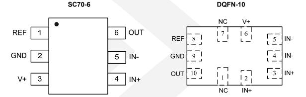
Figure 1 Pin Assignment (Top View)
