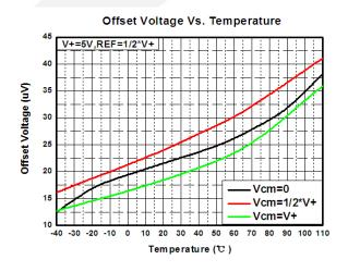
Figure 5. Offset Voltage Vs. Temperature (DIO2399B: 100V/V)
