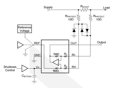
Figure 16. DIO2399x Transient Protection Using a Single Transzorb and Input Clamps
