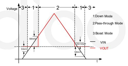
Figure 2 Down Mode and Pass-Through Operation
