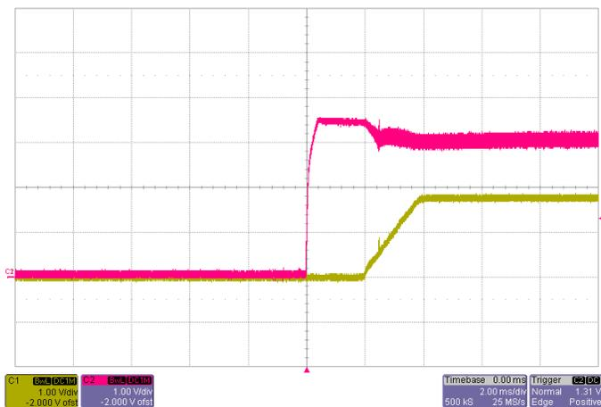
Start-up  $V_{IN}=3.3V$ ,  $I_O=22A$
