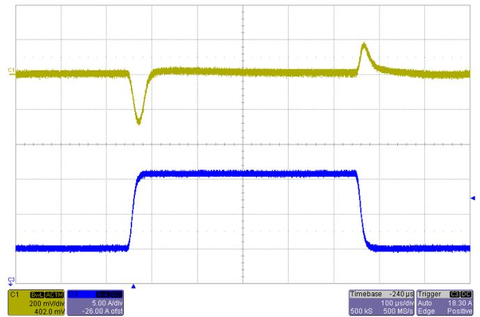
Transient Response  $V_{IN}=3.3V$ , Step from 11A~22A~11A
