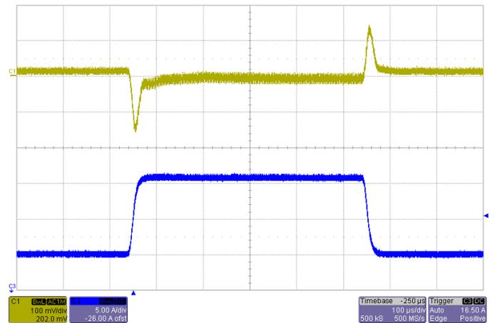
Transient Response  $V_{IN}=3.3V$ , Step from 11A~22A~11A
