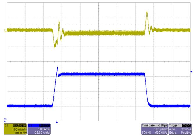
Transient Response  $V_{IN}=3.3V$ , Step from 11A~22A~11A
