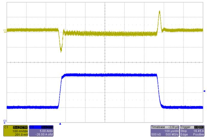
Transient Response  $V_{IN}=3.3V$ , Step from 11A~22A~11A
