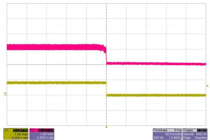
Shut-down  $V_{IN}=3.3V$ ,  $I_O=22A$
