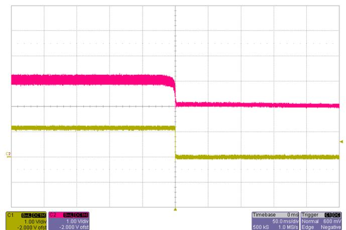
Shut-down  $V_{IN}=3.3V$ ,  $I_O=22A$
