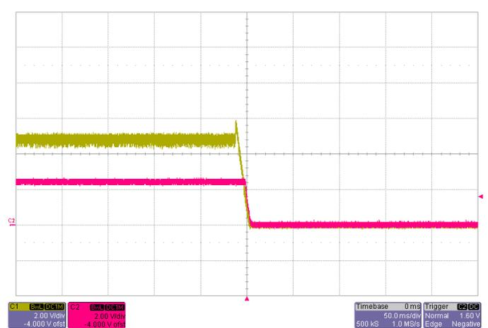
Power Down with Auto-Track Control  $V_{Track}=5.0V$ ,  $I_O=22A$
