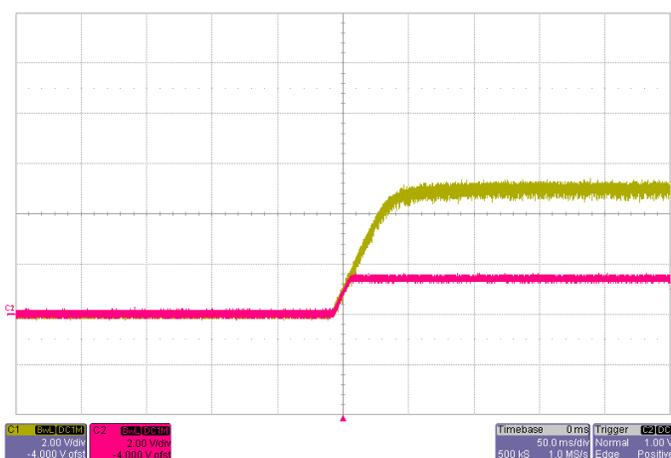
Power Up with EasyTrack™ Control  $V_{Track}=5.0V$ ,  $I_O=22A$
