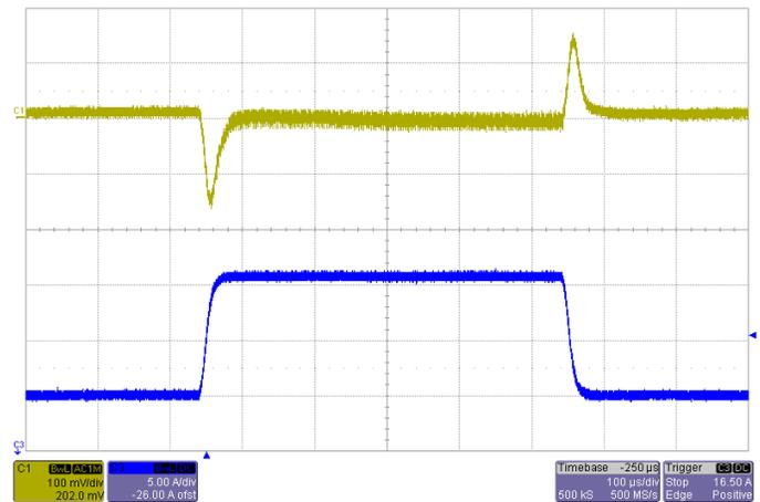
Transient Response  $V_{IN}=3.3V$ , Step from 11A~22A~11A
