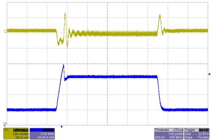
Transient Response  $V_{IN}=3.3V$ , Step from 11A~22A~11A
