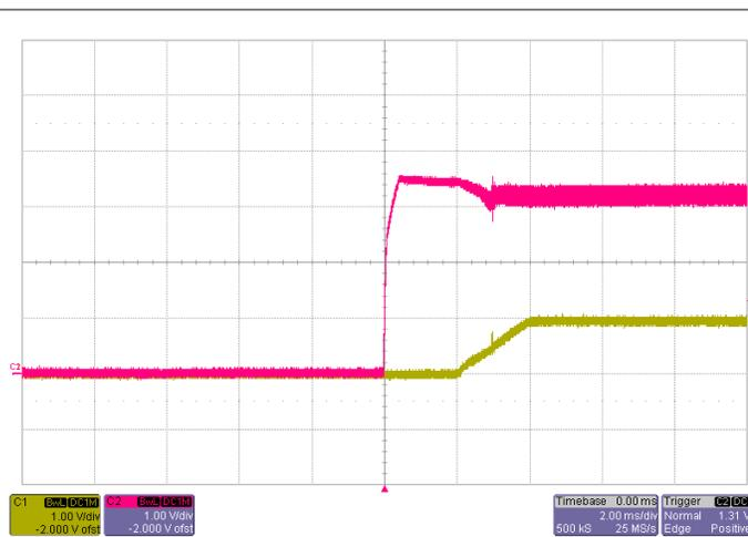
Start-up  $V_{IN}=3.3V$ ,  $I_O=22A$
