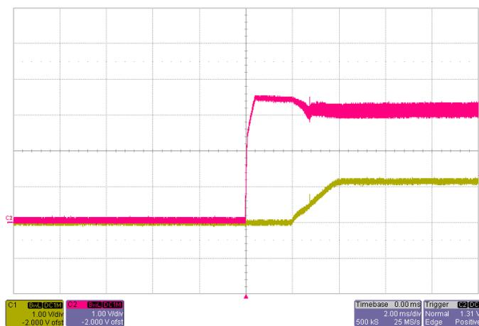
Start-up  $V_{IN}=3.3V$ ,  $I_O=22A$
