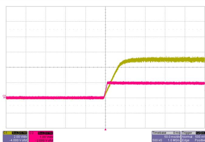
Power Up with EasyTrack™ Control  $V_{Track}=5.0V$ ,  $I_O=22A$
