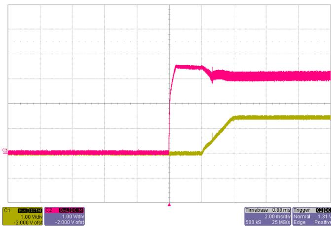
Start-up  $V_{IN}=3.3V$ ,  $I_O=22A$
