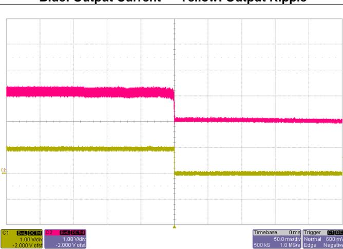
Shut-down  $V_{IN}=3.3V$ ,  $I_O=22A$
