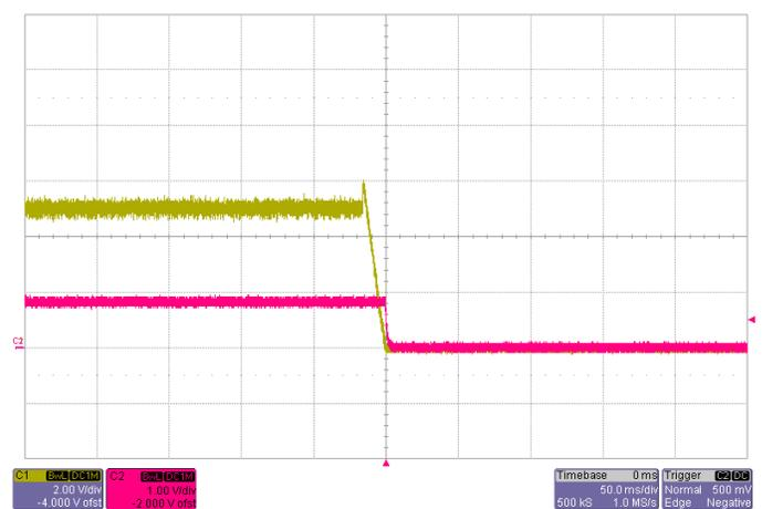
Power Down with EasyTrack™ Control  $V_{Track}=5.0V$ ,  $I_O=22A$
