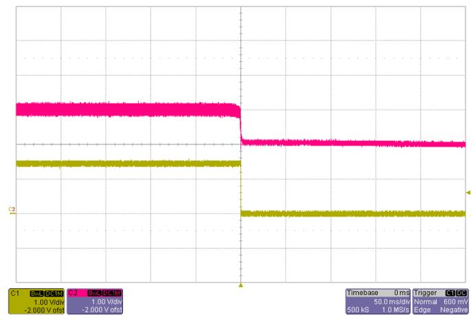
Shut-down  $V_{IN}=3.3V$ ,  $I_O=22A$
