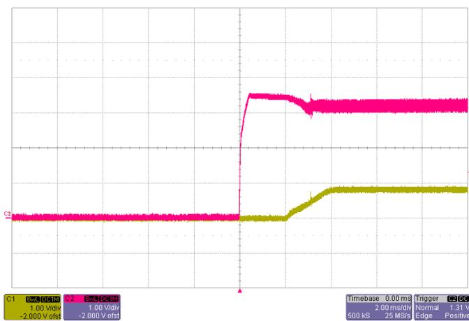
Start-up  $V_{IN}=3.3V$ ,  $I_O=22A$
