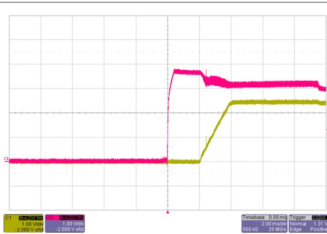
Start-up  $V_{IN}=3.3V$ ,  $I_O=22A$
