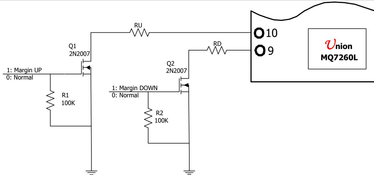
**Fig4 Margin up and Margin down application circuit**
