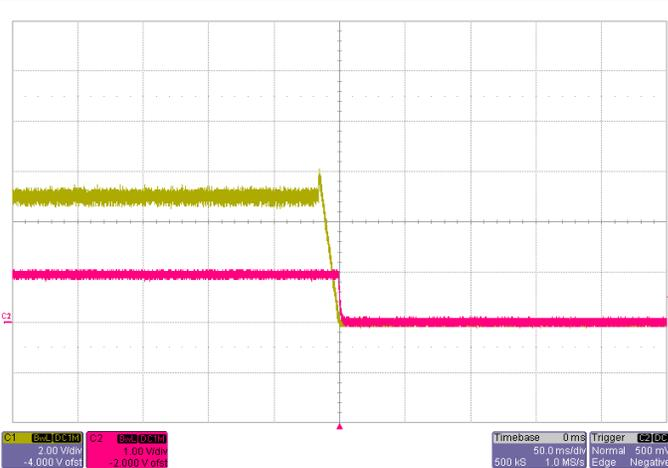
Power Down with EasyTrack™ Control  $V_{Track}=5.0V$ ,  $I_O=22A$
