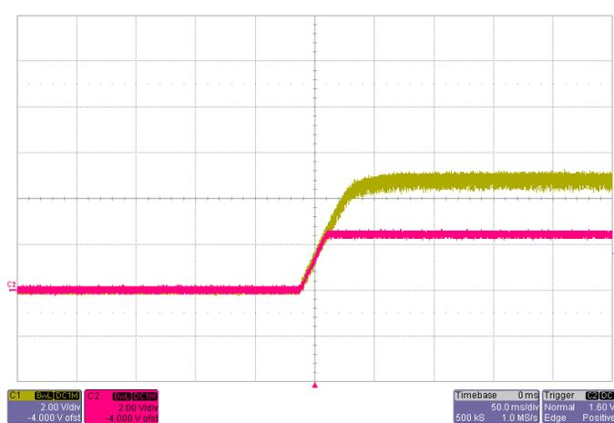
Power Up with Auto-Track Control  $V_{Track}=5.0V$ ,  $I_O=22A$
