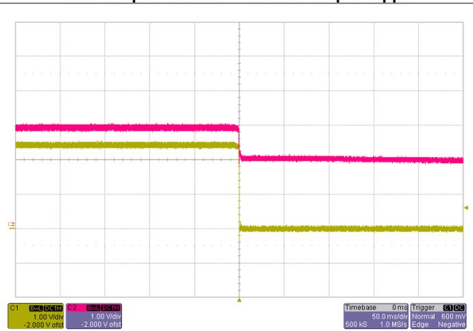
Shut-down  $V_{IN}=3.3V$ ,  $I_O=22A$
